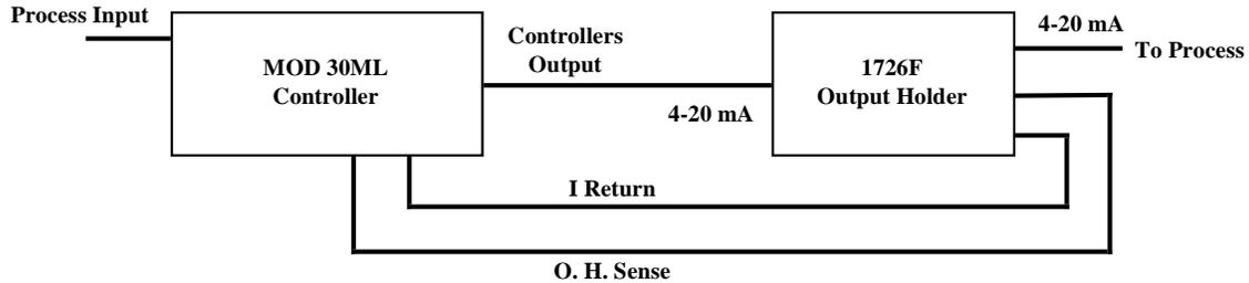
Figure 2. Generic Output Holder Connection Diagram
