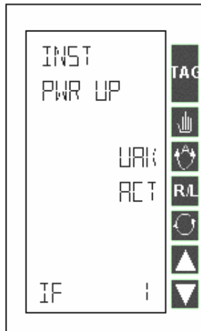
Figure 3 .3. MOD 30ML Alarm CLeaRed Alarm
